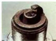
Fig.2 Fouling of spark plug
