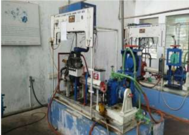
Fig.3:- 4-Stroke, 4-Cylinder Petrol Engine Setup before FTA
