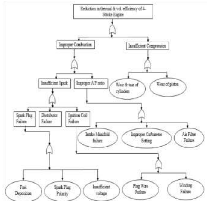
Fig. 1 Fault tree analysis of I. C engine
