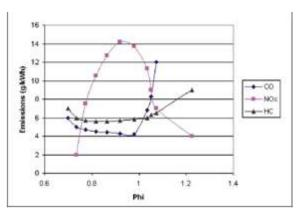
the NOx for a gasoline engine is re-duced as phi decreases (similar to a hydrogen engine). How-ever, in a gasoline engine the reduction in NOx is compromised by an increase in carbon monoxide and hydro-carbons. The theoretical maximum power output from a hydrogen engine depends on the air/fuel ratio and fuel injection method used.
