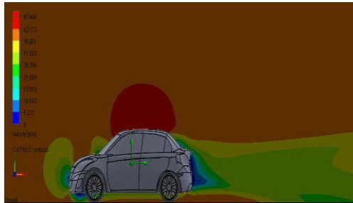
Fig 3.1.b: Velocity Contour without modifications
