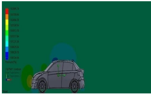
Fig 3.3.a: Pressure Contour with Vortex Generator
