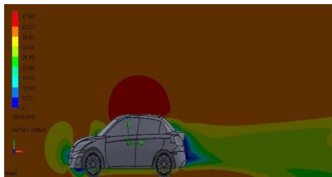
Fig 3.3.b: Velocity Contour with Vortex Generator
