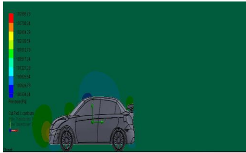
Fig 3.4.a: Pressure Contour with Spoiler
