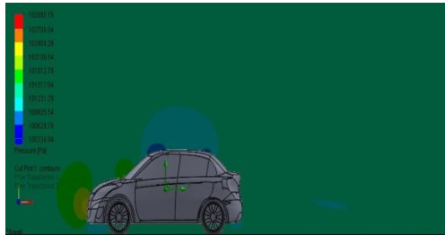
Fig 3.1.a: Pressure Contour without modifications
