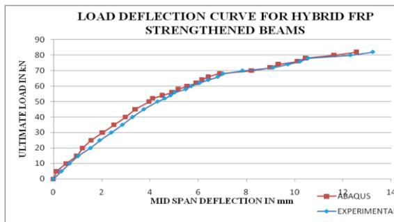
**Figure 5.2 Load deflection curves for strengthened beams, obtained by Experimental and Abaqus model**
