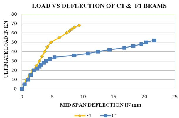
**Figure 4.1 Load deflection curve for F1 beams**
