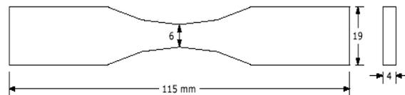
The specimen is loaded in universal testing machine. Specimens were fixed in the upper jaw first and then gripped in the movable jaw (lower jaw). Initially strain was kept at zero. The load as well as the extension was recorded digitally with the help of a load cell and an extensometer respectively. From these data, stress strain curve was plotted; the initial slope of which gives the young's modulus. The ultimate stress and ultimate load were obtained at the failure of the specimen.
