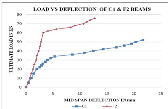
Figure 4.2 Load deflection curve for F2 beams
