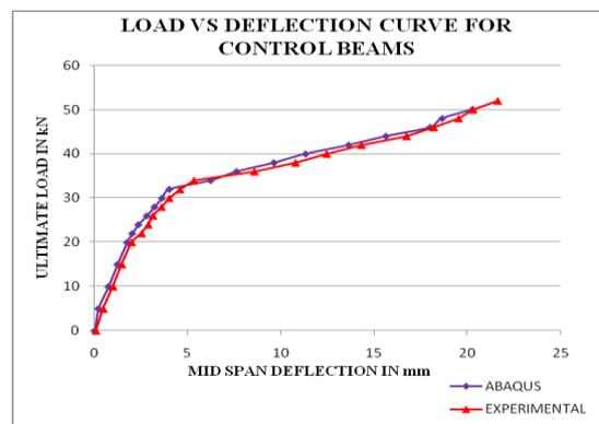
**Figure 5.1 Load deflection curves of control beams, obtained by Experiments and Abaqus model**
