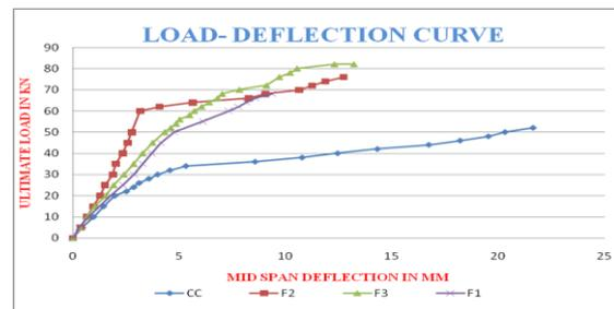
Figure 4.4 Load deflection curve for beams F1, F2, F3
