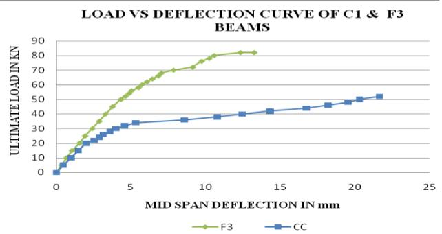
Figure 4.3 Load deflection curve for beams F3
