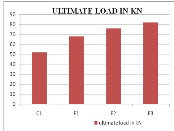
**Figure 4.6 Ultimate crack loads of the beams**
