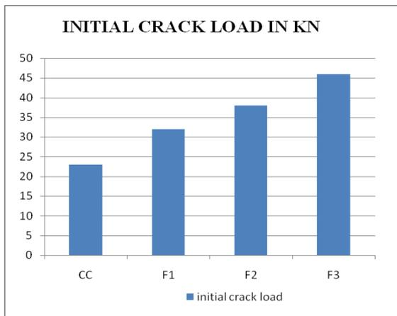
**Figure 4.5 Initial crack load of the beams**
