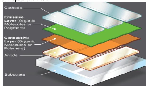
Fig 1.2: OLED layers
