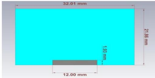
Fig. 1 (c) Spinal view of the propounded antenna design.
