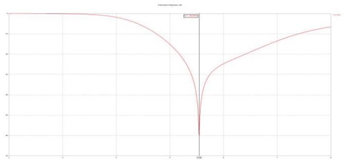
Fig. 2(a) Return loss (S11) showing resonant frequency of antenna design.
