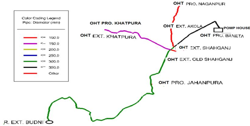
Fig.1 Clear water feeder network phase 1 Baneta
