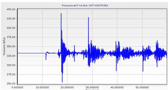
Figure-8 Pressure at pipe P-14 connected to Khatpura for valve closure time 5 sec
