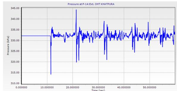
Figure-9 Pressure at pipe P-14 connected to Khatpura for valve closure time 10 sec
