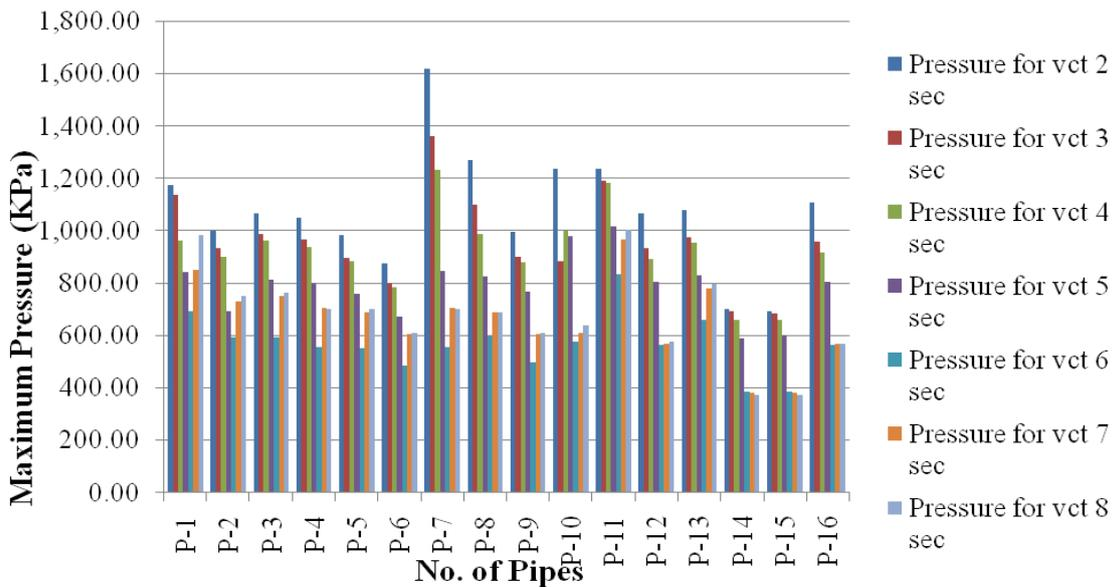
Fig.-5 Maximum Pressure in different pipes at different valve closure time in Feeder network Phase-1
