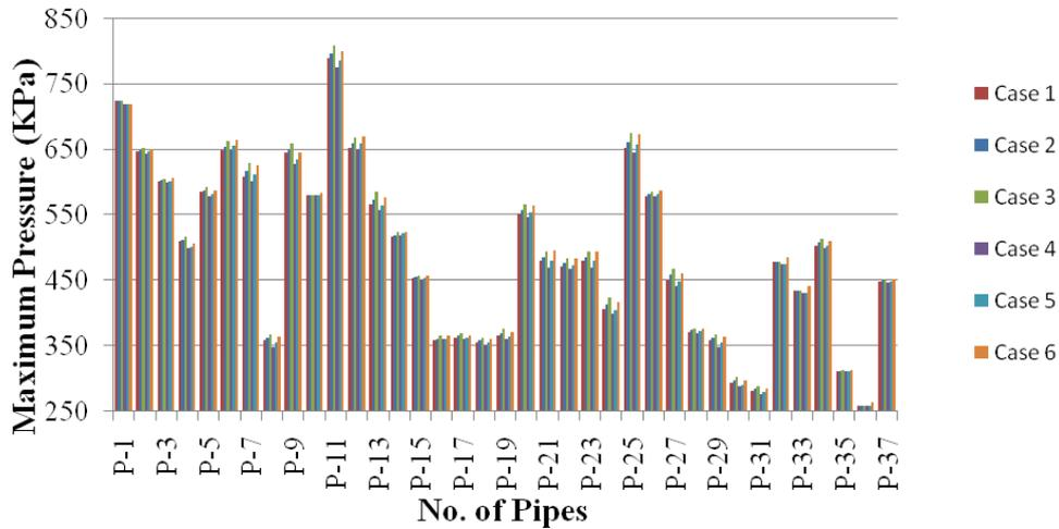
Fig.-4 Maximum pressure in different pipes due to change in pump inertia in Feeder network Phase-2
