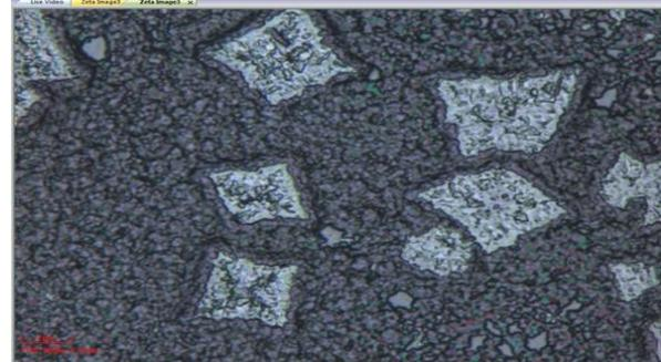
**Fig.11(b)** Glass plate was covered on boat to prevent evaporation, Substrate= glass/ 5 nm Al by evaporation, Solute concentration= 55.4 wt%  $\text{ABl}_3$  in DMF, Amount of solution = 50  $\mu\text{l}$ , Substrate temp. = 100  $^\circ\text{C}$ , Deposition time = 45 min, annealing time = 15 min.
