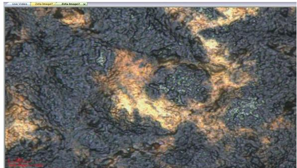
**Fig.11(j)** Substrate= glass/ 70 nm Al, Solute concentration= 4.77 wt%  $\text{ABI}_3$  in DMF, Amount of solution = 30  $\mu\text{l}$ , Deposition time = 35 min, Solution was kept on substrate only and didn't allowed to pour below substrate.
