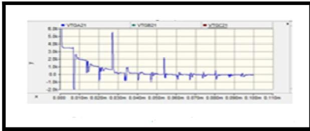
Fig. 8: Phase Voltage with Back Flashover
