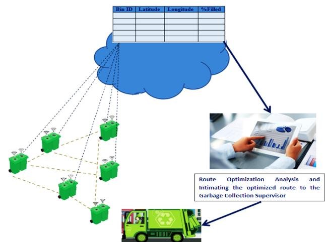
**Fig1.Overall System Block Diagram**
