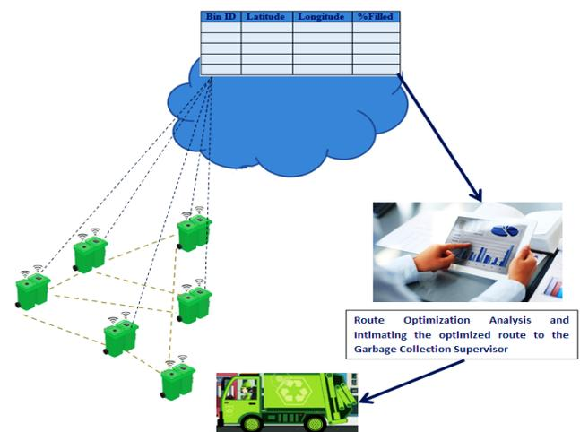
**Fig1.Overall System Block Diagram**
