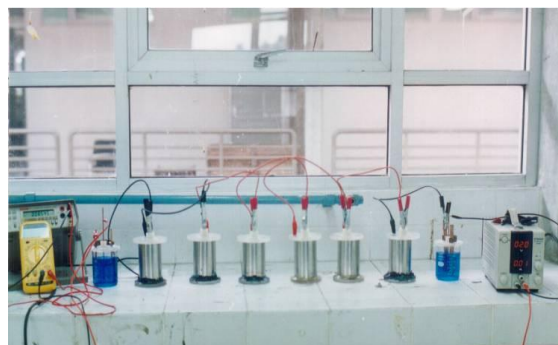
Fig. 3 Galvanostatic experiment for anode of Mg
