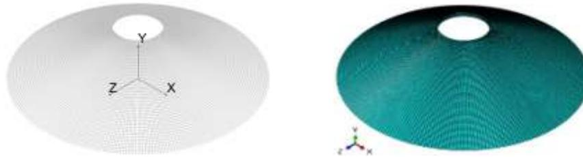
Fig. 4 Mesh structure of the models in Cosmos/M (on the left) and Abaqus (on the right).
