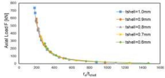
Fig. 11 F vs.  $r_e/t_{shell}$  curves for the results of Abaqus
