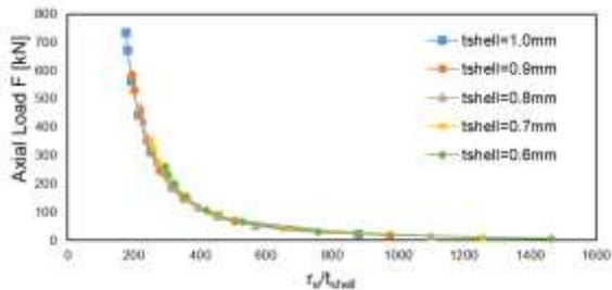
Fig. 10 F vs.  $r_e/t_{shell}$  curves for the results of Cosmos/M
