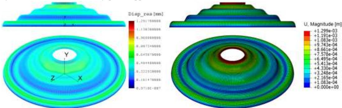
Fig. 6 F – Deformed shapes from Cosmos/M (on the left) and Abaqus (on the right). (Deformation scale factor = 20)
