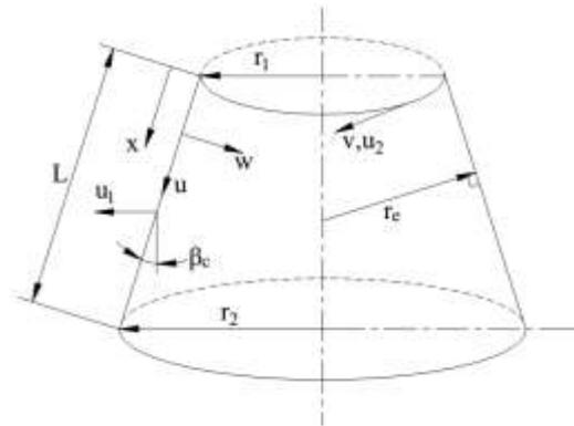
Fig. 2 Basic truncated conical shell geometry and notations [7].
