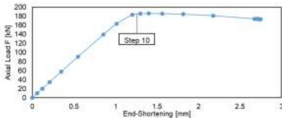
Fig. 5 F – End-shortening curve obtained from Abaqus for  $\beta_c = 60^\circ$  and  $t_{shell} = 1mm$ .
