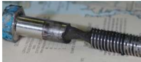
Fig. 4 Crevice corroded stainless steel [26]
