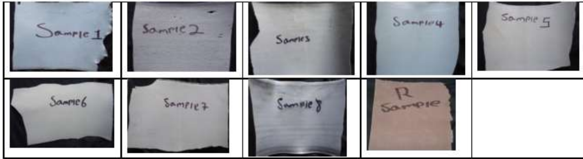
Fig2. Photograph 2 sheet samples: Sheet form of EVA/LDPE/Additives produced for prosthetic and orthotic application and R- The reference EVA used for prosthetic and orthotic application in Addis Ababa medical faculty Black lion hospital
