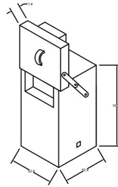
Fig 2: Isometric sketch of the furnace
