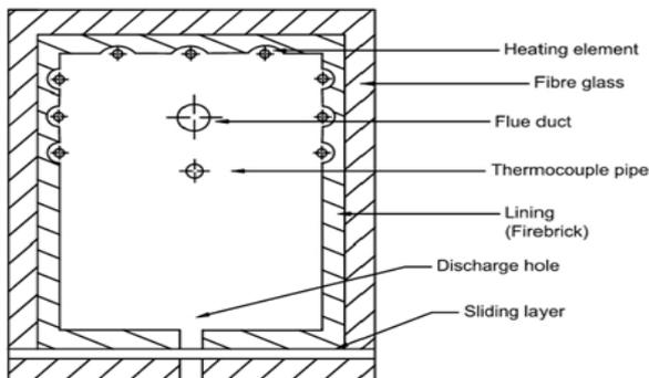
Fig 1: Sectional Drawing of the furnace
