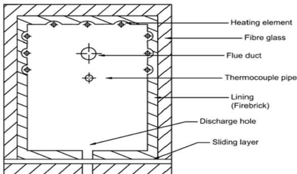
Fig 1: Sectional Drawing of the furnace
