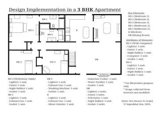
In this implementation, we need 35 switches i.e. 35 relay modules. A standard relay PCB (Printed Circuit Board) can contain up to 16 relays but we will be using 8-relay PCBs for easy implementation. So, we need:
