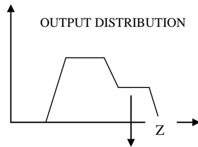
Fig. 3 Defuzzification based on the Center of Mass
