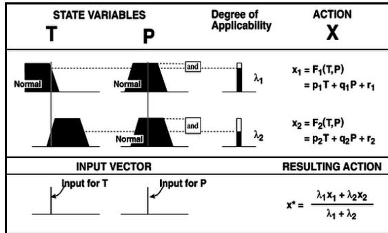
Fig. 5 Sugeno FIS for two Input values
