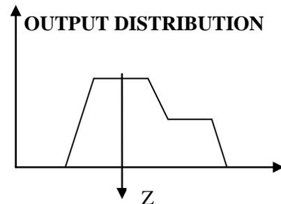
Fig. 4 Defuzzification based on the Mean of maximum
