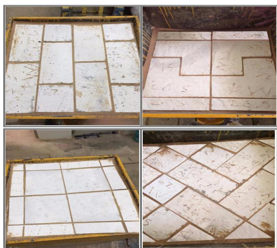
Figure (4) Various shapes of pavers and laying patterns
