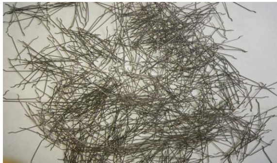
Fig.1 used Hooked end steel fibers in the study Mix design carried out by using ACI:211.4R –93 (Reapproved 1998) method. The mix proportion obtained for plain M50 grade concrete is 1:1.41:2.56:0.007(SP) with water – cement ratio 0.32 .
