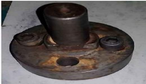
Figure 4: Induction Hardening Fixture
