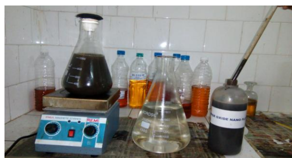
Figure(5): Magnetic stirring of water dispersion nano fluid
