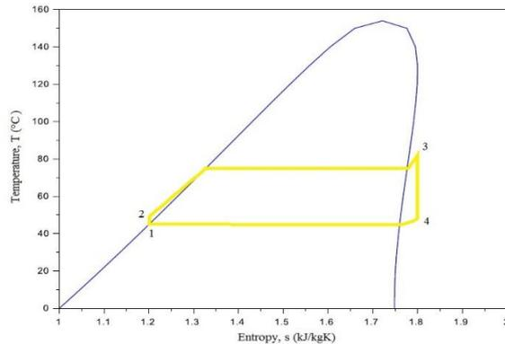
Fig 11: A subcritical ORC having R245fa as the working fluid
