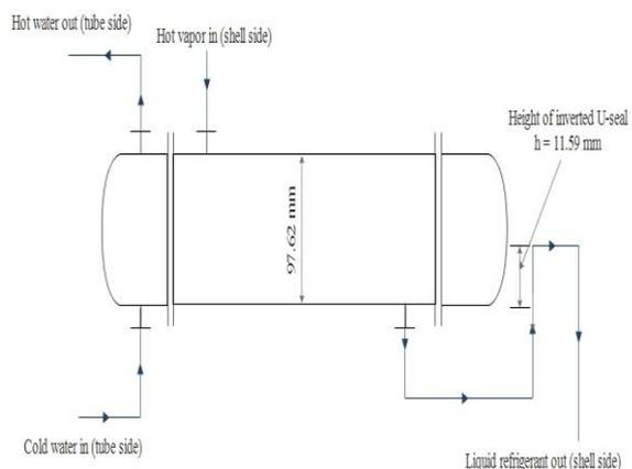
Fig 8: Diagram of the shell and tube condenser
