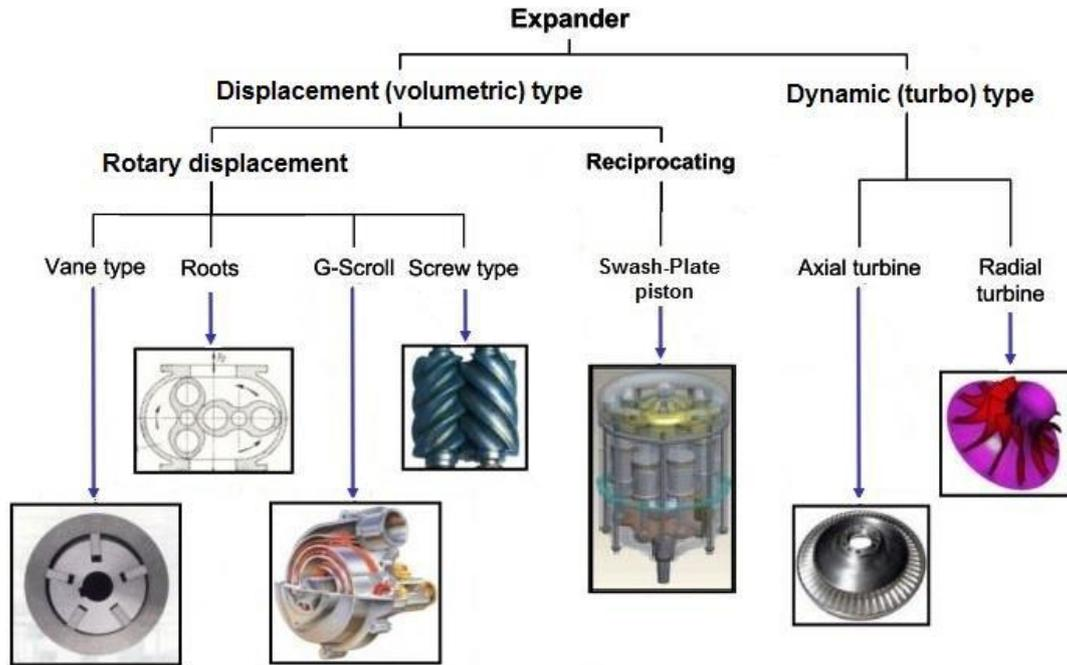
Fig 2: Diagram of the various expander types [5]
