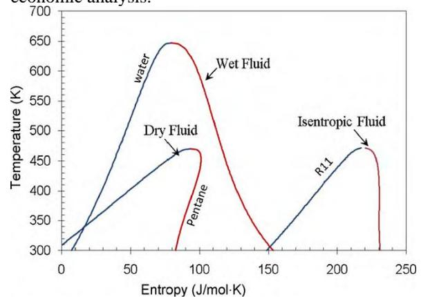
Fig 3: Three types of working fluids- dry, isentropic and wet [6]
