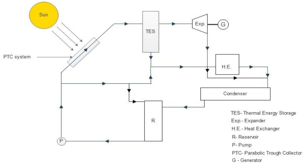
Fig 1: Block diagram of the ORC system
