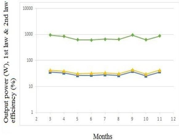
**Fig 9 Expander Output Power in kW (green), 1<sup>st</sup> law efficiency in % (blue), 2<sup>nd</sup> law efficiency in % (yellow) vs. corresponding months**
