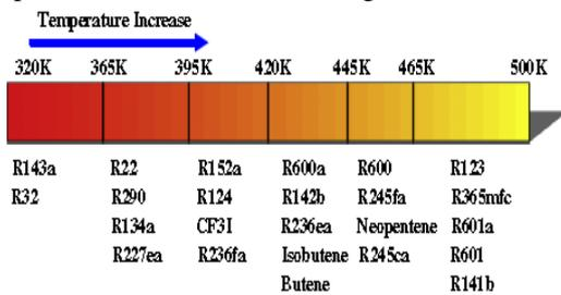
**Fig 4: The optimal selections of working fluids corresponding to the heat source temperature level [6]**
