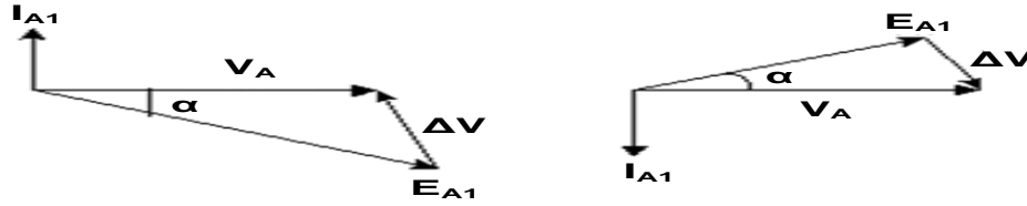
Figure 2b: Leading and Lagging power factor characteristic phasor diagram
