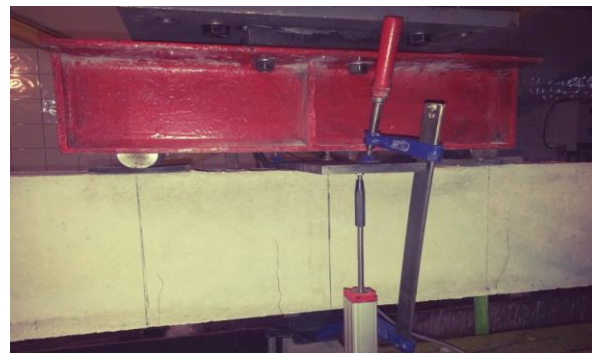
Fig 9: Crack in prestressed SFRC.
