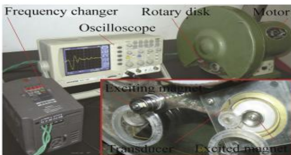
Fig. 16: Piezo-disk energy harvester excited by rotary magnets (PEHRM) [6]
