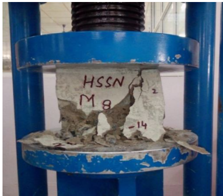
Fig 2: Compression test on Concrete cube (After load is applied)
