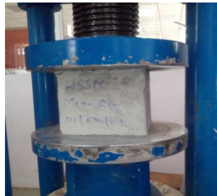
Fig 1: Compression test on Concrete cube (Before load is applied)
