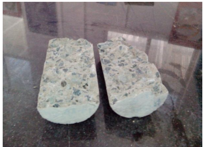
Fig. 4 (b) cylinder after tensile test
