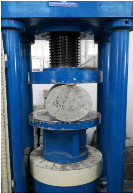
Fig 6: Tensile strength test on Concrete cylinders
