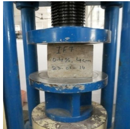
Fig 2: Compression test on Concrete cube
