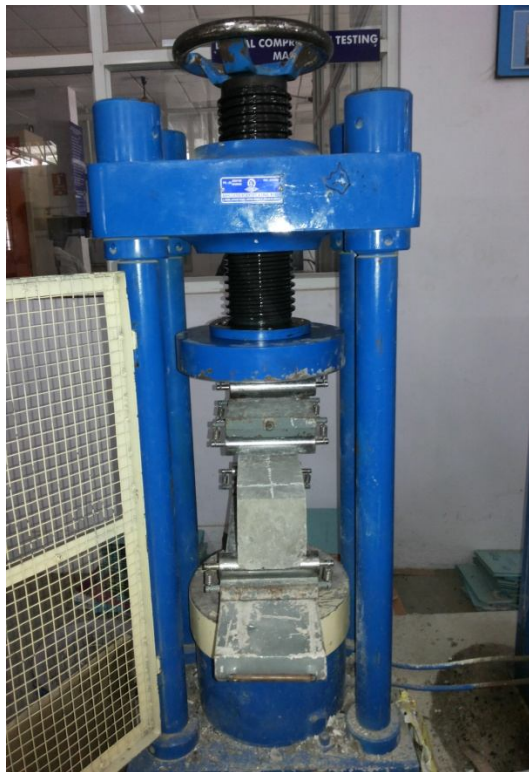
Fig 10: Flexure strength test on Concrete beams
