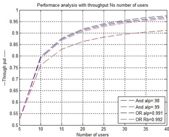
Fig. 7: Throughput versus the number of users for a fixed  $\alpha$ .
