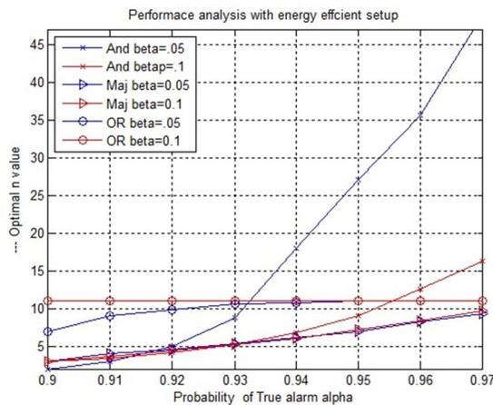
Fig. 4: optimal  $N$  versus the probability of detection constraint for the energy efficient setup.
