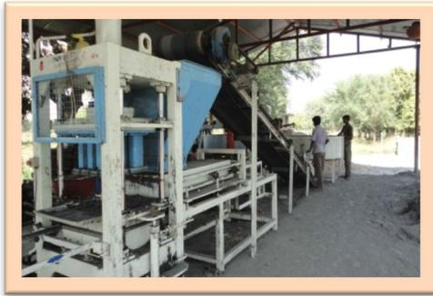
**FIGURE 4: SET UP OF AUTOMATIC FLY ASH BRICK PLANT**
