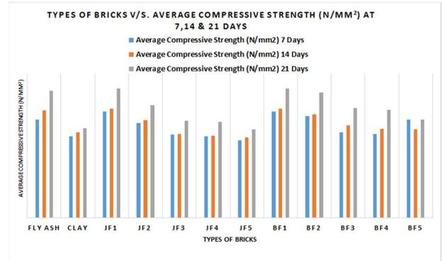
FIGURE 8: TYPES OF BRICKS V/S AVERAGE COMPRESSIVE STRENGTH (N/mm<sup>2</sup>) AT 7, 14 AND 21 DAYS
