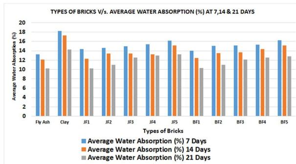
**FIGURE 11: TYPES OF BRICKS V/S AVERAGE WATER ABSORPTION (%) AT 7, 14 AND 21 DAYS**
