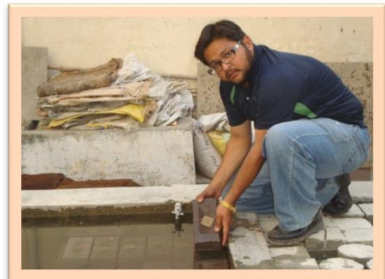
FIGURE 10: CURING OF SAMPLE BRICK
